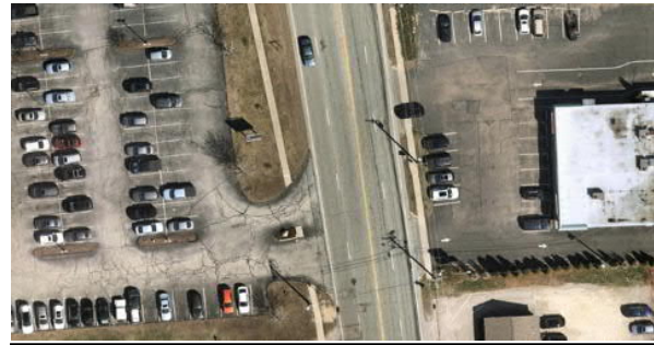
Sidewalk not continued through driveway at 324 Flanders Road. Wide curb cuts at 323 Flanders Road.
